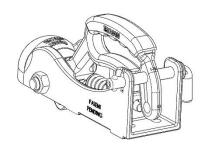
The lock barrel can be fitted to the end of the safety lock pin as shown. Use the rubber cap provided over the end of the lock barrel to prevent ingress of contaminants.
